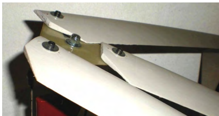
Wooden blades of the author, covered with thermoretractable film.
